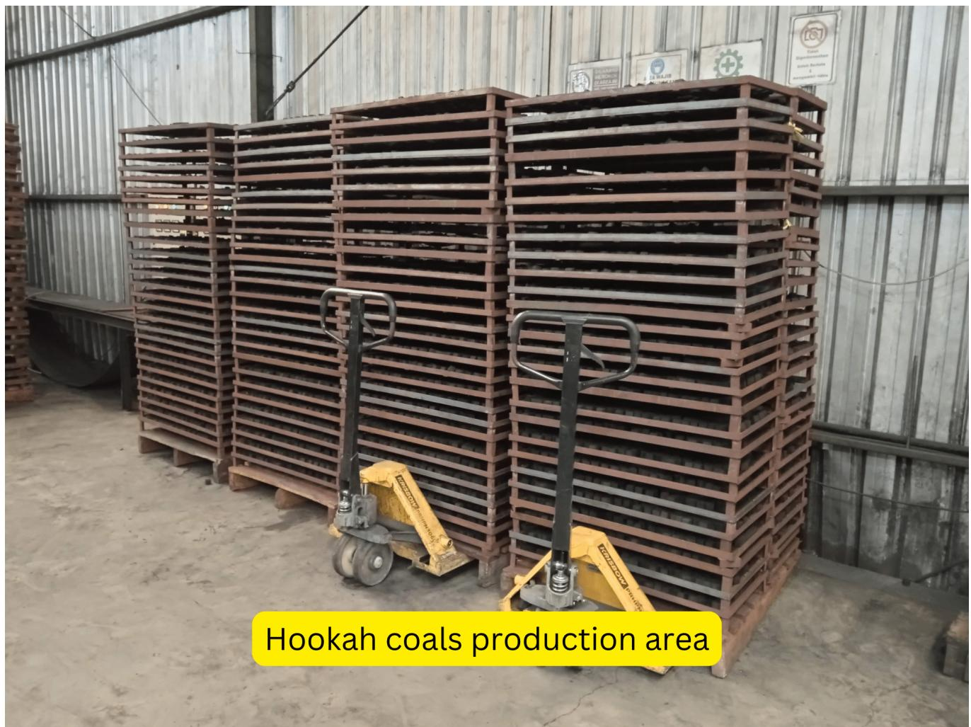
Ok, production consist from grinding charcoal – making it is into small mesh, like a flour, that we use for cooking. Then we mixed it with tapioca. Tapioca is natural stretch that make coconut charcoal briquettes strong and not crack or fall down during the shisha smoking.
