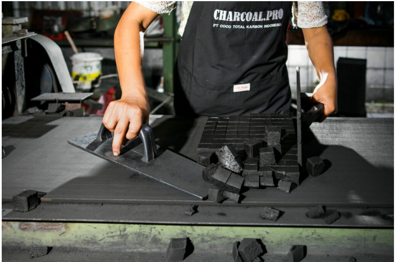
Production of coconut shell charcoal briquettes for hookah
