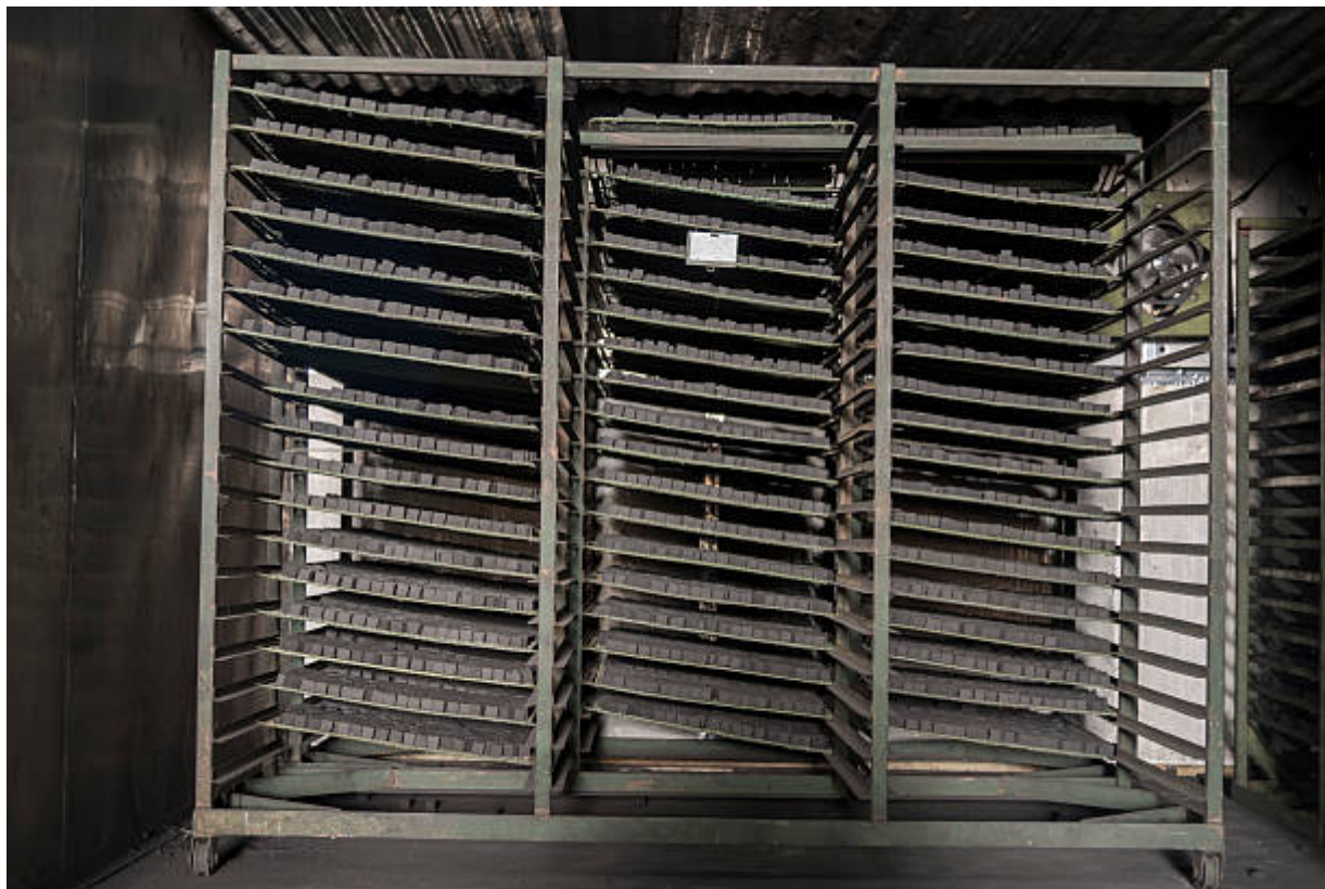
charcoal.pro coconut charcoal production drying process
